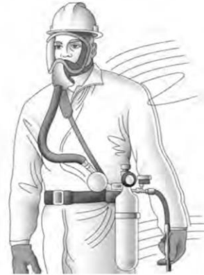
Full Facepiece Supplied-Air Respirator (SAR) with an auxiliary Escape Bottle APF=1,000 APF = 10,000 (if used in "escape" mode) Needs to be fit tested
